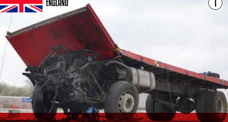
SHALLOW MOUNTED BOLLARD 7500 KG / 80 KM
