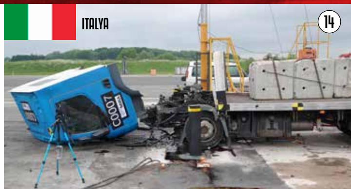
COUNTER TERROR FOLDING BOLLARD 7200 KG / 48 KM
